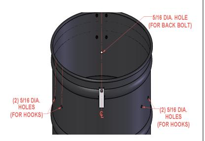
LAYOUT MARK AND DRILL (5) 5/16" DIA. HOLES PPROXIMATELY 8" DOWN FROM DRUM TOP LIP. THE HOOK MOUNTING HOLES SHOULD BE ON APPROXIMATELY 3 1/4" CENTERS.
