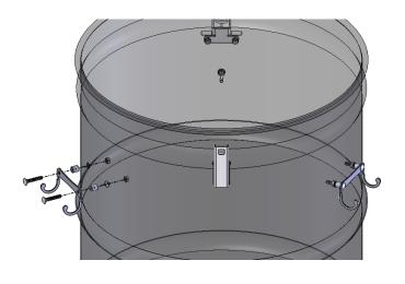
MOUNT THE HOOKS WITH THE SPACERS AND THE BACK CENTER BOLT TO THE DRUM. THE (5) 1-1/2" LONG BOLTS WILL BE USED TO SUPPORT THE COOKING GRATE.
