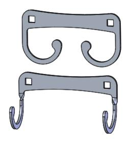
WITH ADJUSTABLE WRENCH OR PLIERS, TWIST THE (2) HOOKS OUT APPROXIMATELY 90 DEGREES. (2)
