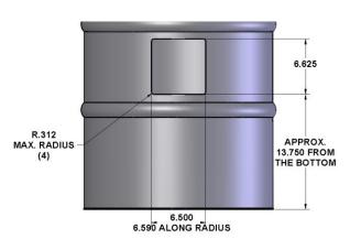
DETERMINE CUTOUT LOCATION FOR THE CHARCOAL CHUTE. LAYOUT AS SHOWN ABOVE. AND CAREFULLY CUTOUT.
