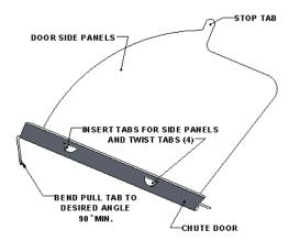
INSERT DOOR SIDE PANELS INTO CHUTE DOOR SLOTS AND TWIST TABS (4) TO ATTACH. BEND DOOR PANELS OUT, TO KEEP PANELS FROM FALLING IN ON THEMSELVES. BEND PULL TAB DOWN TO DESIRED ANGLE.
