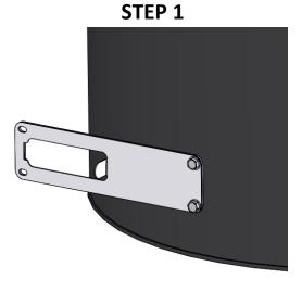
MOUNT INLET (ALL (3) PIECES) APPROXIMATELY 2" FROM BOTTOM. USING 3/8" HEX DRIVE ASSEMBLE (2) SELF-DRILLING SCREWS ON ONE END WHILE BENDING THE (3) PIECES AROUND THE DRUM, INSTALL THE OTHER (2)
