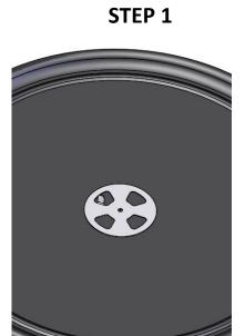
LAY EXHAUST VENT ON TOP OF LID IN LOCATION FOR MOUNTING. MARK THE CENTER HOLE AND THE (4) OTHER OPENINGS. REMOVE EXHAUST VENT
