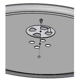
DRILL 5/16" HOLE FOR THE CENTER PIVOT HOLE. AND DRILL (4) 5/8" TO 3/4" DIA. HOLES IN THE APPROXIMATE MIDDLE OF THE OTHER MARKINGS. INSTALL BUTTON HEAD SCREW AND LOCK NUT.
