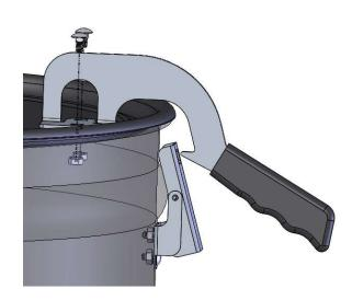
PLACE HANDLE ON LID. MAKE SURE LATCH WILL DISENGAGE THE HANDLE HOOK AND MARK THE (2) MOUNTING HOLES REMOVE HANDLE AND DRILL (2) 5/16" DIA. HOLES AND MOUNT HANDLE TO LID WITH (2) CARRIAGE BOLTS AND (2) LOCK WASHER NUTS.
