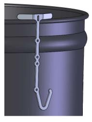
PLACE (OPTIONAL) TEMPLATE/HOOK ON DRUM LIP AND MARK THE (2) MOUNTING HOLES FOR LATCH. REMOVE TEMPLATE AND DRILL (2) 5/16" DIA. HOLES. SEE **STEP 2A** IF YOU DON'T HAVE THE (OPTIONAL) TEMPLATE/HOOK.
